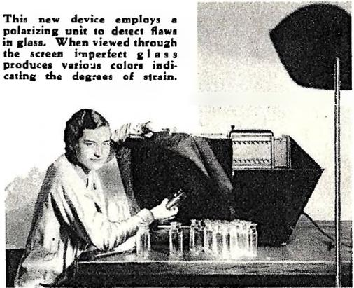
**S**TRAINS in glass or any other transparent or semi-transparent object, are made visible by a new optical instrument consisting of a polarizing unit and an analyzing unit.
