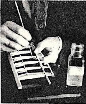
Gluing in the angle braces used to strengthen wing ribs at points of attachment for the bracing wires. Leading edge has been sanded and wing is ready for covering.
