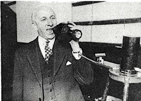
Equipped with one of these photo cell telephones you can talk to a neighbor without being connected by wires. The electric impulses travel over a light beam instead of telephone wires.
