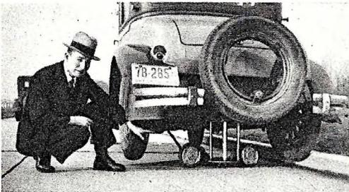
This unique car parker operates from the automobile motor. An auxiliary gear shift raises the car on the jack, swings it left or right, and lowers it into position by the curb.
